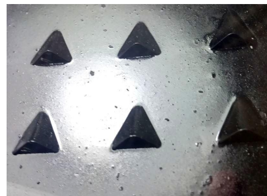
Fig. 2 (a) Schematic of the protruding triangular openings on the absorber plate and the air flow around them (b) photograph of the openings
