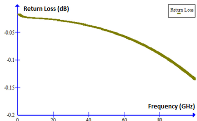
Fig. 9. Return loss in off state.
