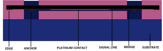
Fig. 5. Figure showing cross section of the bridge.
