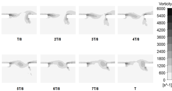
Fig. 6 Instantaneous vorticity contour for one period
