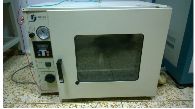
FIG. 11. Furnace for glass thermal slumping.
