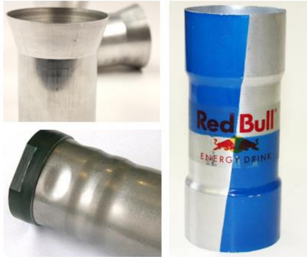
Fig. 9 Example of expansion and compression[8]
