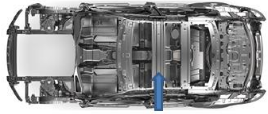
Fig. 1 A typical rail roof center member
