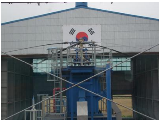
Fig. 10. Whirl tower test of BMR
