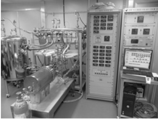
Fig. 3 A experimental apparatus of a DU bed 1)
