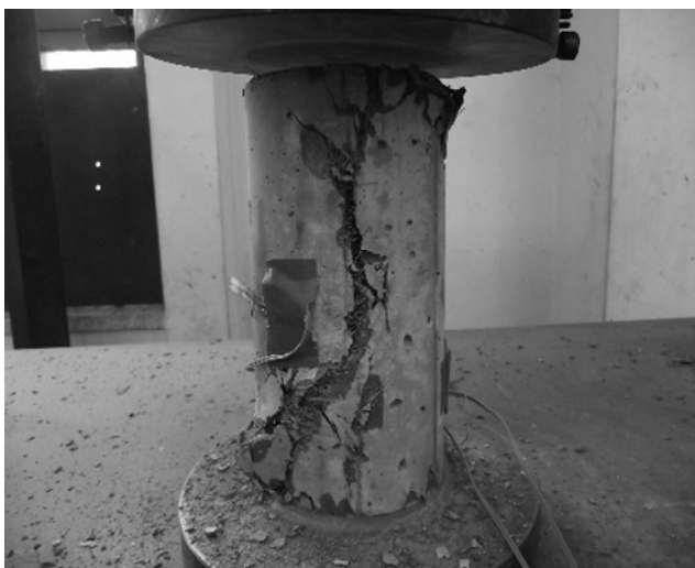
Fig. 5 Typical failure mode of UHPC ( V_f=2\% )
