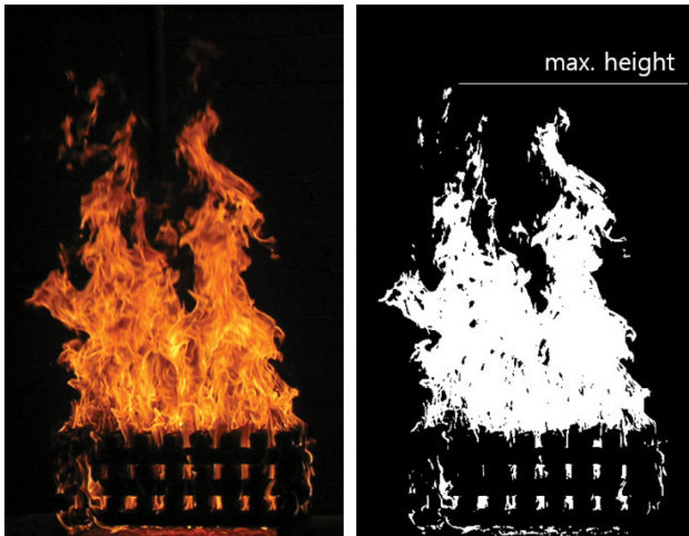
Figure 1. Binary image processing to determine flame height for a wood crib fire.
