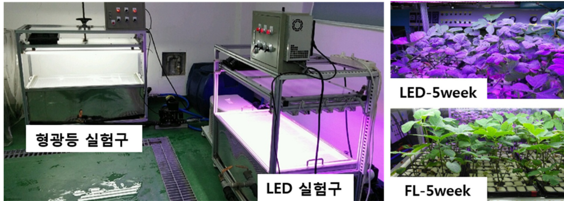
Fig. 1. Photos of culture systems and Angelica gigas growing under the LED and fluorescent lamp (FL) with a hydroponic culture system for 5 weeks.
