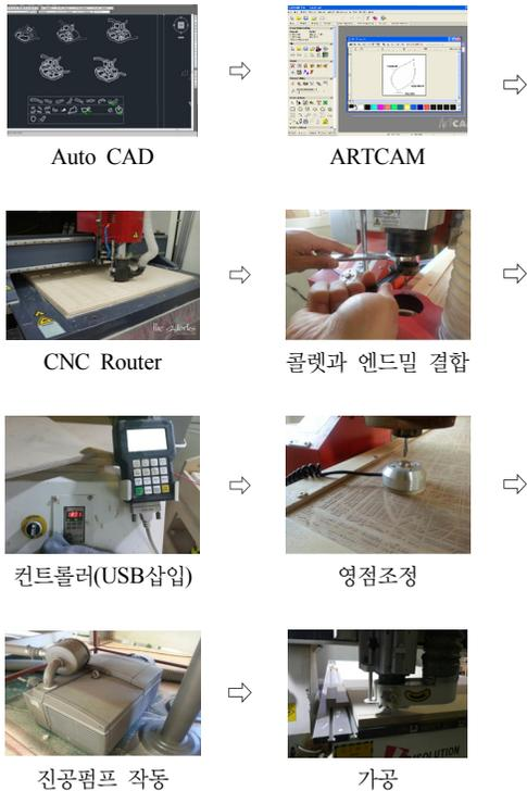
**Fig. 3.** CNC router processing order.
