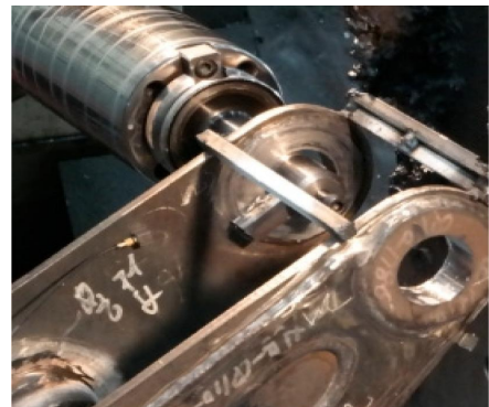
Fig. 5 Cutting process on previous facing tool
