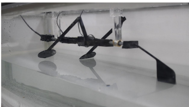
Fig. 1 Water running robot and a tail for enhancing stability
