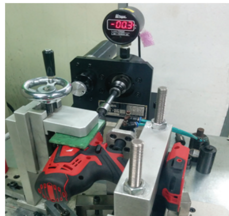
Fig. 5 Measurement device configuration for working torque test
