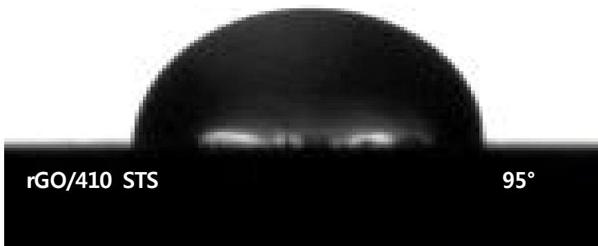
Fig. 16. Water droplet contact angle measurements on (a) bare 316L stainless steel, (b) graphene coated 316L stainless steel, (c) bare 410 stainless steel and (d) graphene coated 410 stainless steel.
