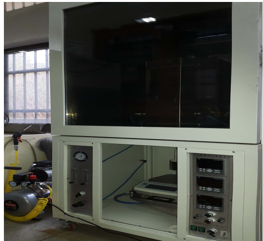
Photo. 1. Apparatus for heat decomposition and combustion gas analysis.
