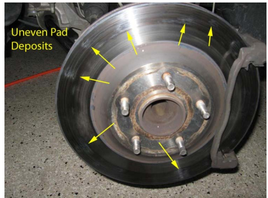
Fig. 2.3. Disc formation by uneven Pad Deposits.
