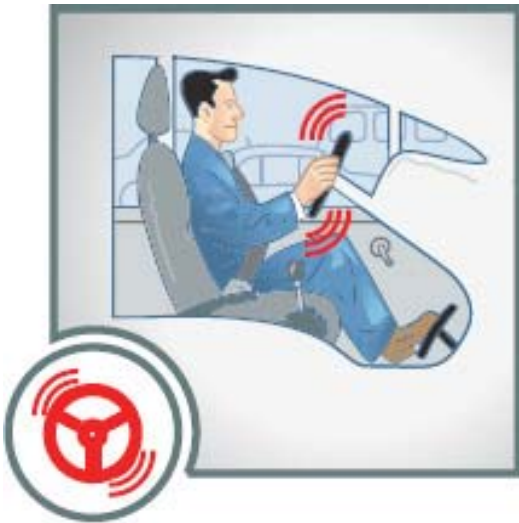
Fig. 2.5. Handle Vaibration by Brake Judder.
