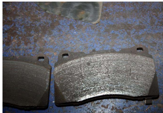
Fig. 3.1. Temperature abrasion of Disc Pad.
