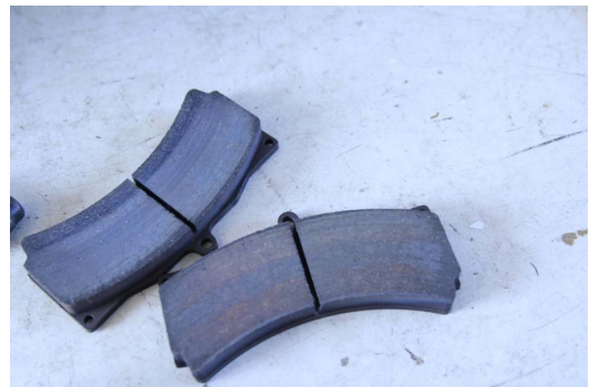
Fig. 2.4. Abnormal wear of Disc Pad.
