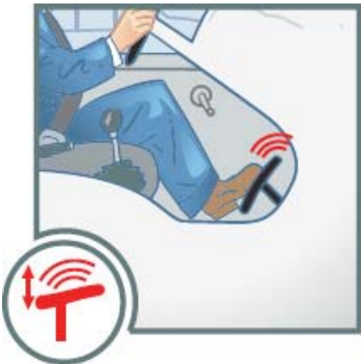
Fig. 2.6. Shuddering of Brake Pedal by Brake Judder.
