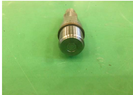
Fig. 13. Pressure measurement sensor and diaphragm device.
