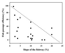
Fig. 2. Scatter plots showing the fish passage efficiency in relation to fishway slope (Redrawn from Noonan et al. 2012). In the plot, " $\diamond$ " indicates the data of Juksan Weir.
