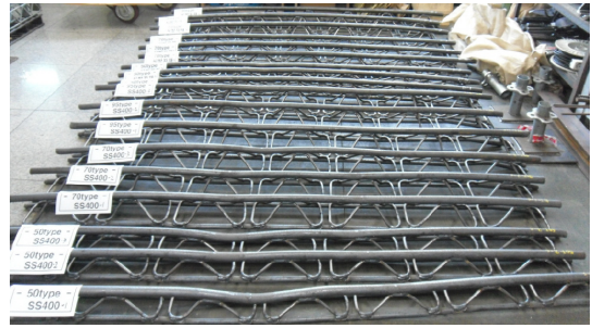
Fig. 6. The specimen after bending test
