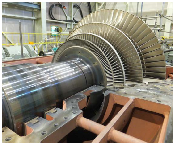
Fig. 2 Photograph of the four-stage low-pressure test steam turbine
