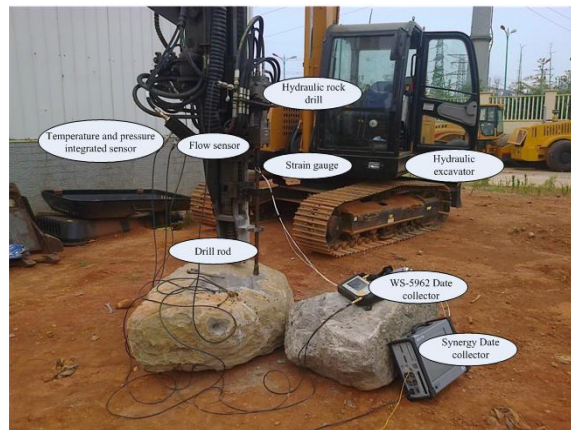
Fig.4 Test system of high frequency hydraulic rock drill drifter
