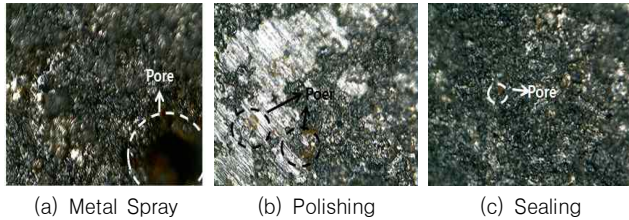
Figure 16. Digital microscope analysis result (× 160)
