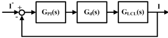
Fig. 2. Block diagram of current control with LCL filter.
