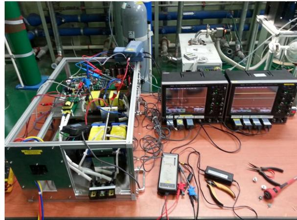
Fig. 14. Test of plasma discharger.
