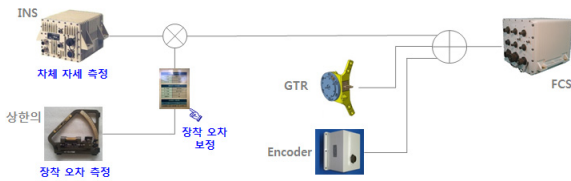
Fig. 11. Compensation for the mis-alignment of INS installation
