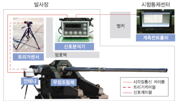
Fig. 1. Composition of muzzle velocity radar system
