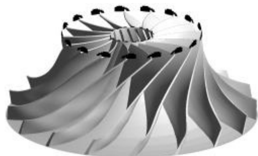
(c) Modified impeller (8.264 kg/s)
