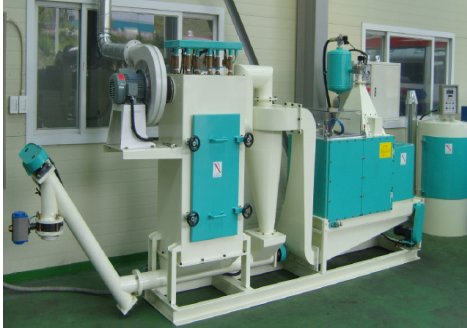
Fig. 2. DPF Cleaning System(Air blowing)
