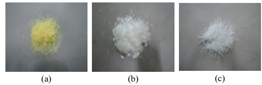
Fig. 1. Shape of PVA and PP-macro (a) RF4000 (b) RSC15 (c) PP-macro
