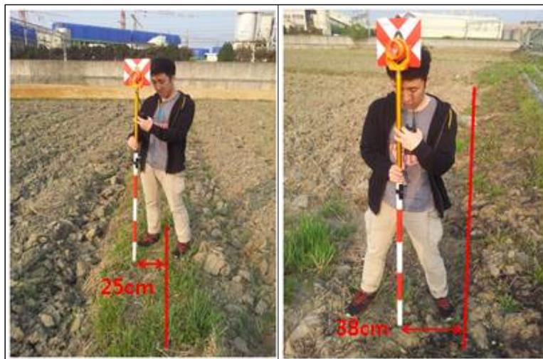
FIGURE 6. Resurveying for verifying the boundary change
