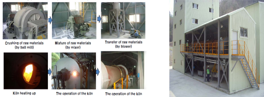
Fig. 3. Green cement pilot plant.
