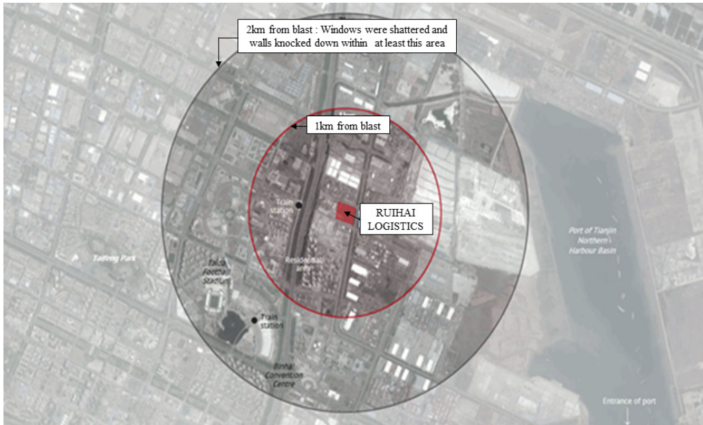
Fig. 2. Damaged boundary by the Tianjin explosion.
