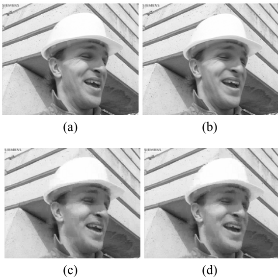
Fig. 6. Original: (a) frame 11 th ; (b) frame 12 th of 'Foreman video'; (c) Decoded 11 th frame (SSIM=0.9313, CR=73.17); (d) Decoded 12 th frame (SSIM=0.9290, CR=65.93)
