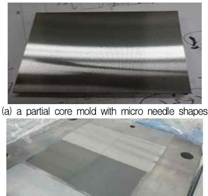
(a) a partial core mold with micro needle shapes
