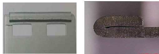
Fig. 11 Hemming shape at 3 stops straight type
