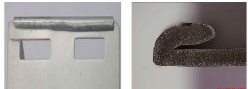
Fig. 10 Hemming shape at 2 steps straight type
