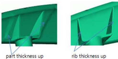
Fig. 2 Product portion changed to part and rib thickness
