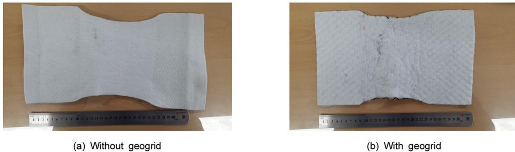
Fig. 2. Results of wide-width tensile test on non-woven geotextiles
