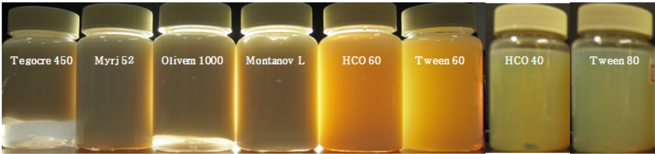
Figure 1. Photograph of nano-emulsions of hydrophilic surfactant / hydrophobic surfactant / candelilla wax / RS White / water system using PIC emulsification process.
