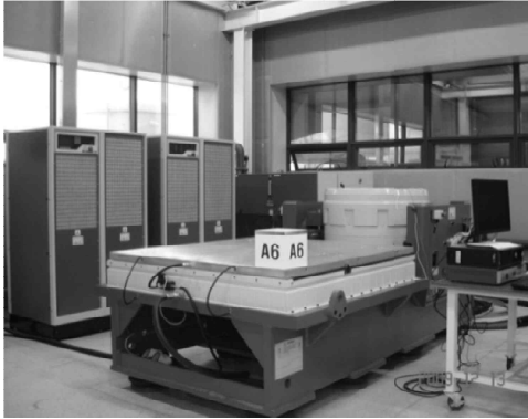
Fig. 8 V9-440-HBT1500C 176K vibration experiment device
