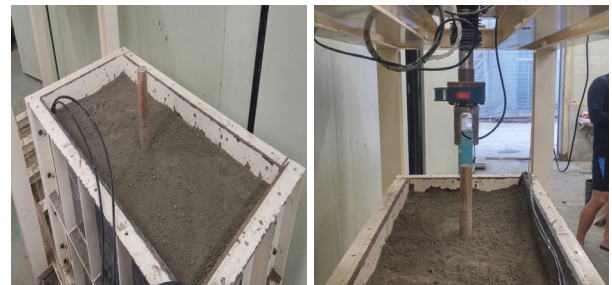
(c) Embedded of pile
