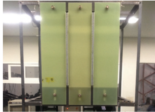
Fig. 6 Set up View of Viscoelastic Damper
