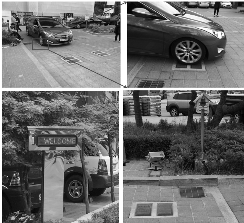
Fig. 13. Field Test of Improved Energy Blocks Under Passing Vehicle
