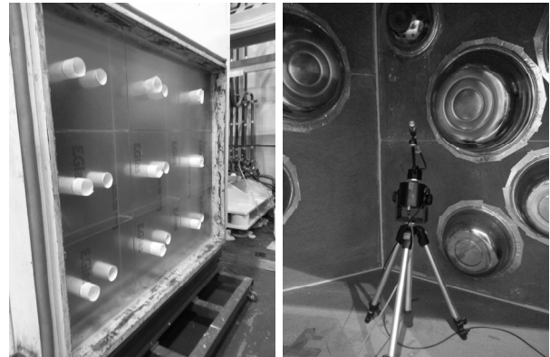
(a) Air Transparent Soundproof Plates with Filters (b) Inside of the Mini-Chamber with A Microphone
