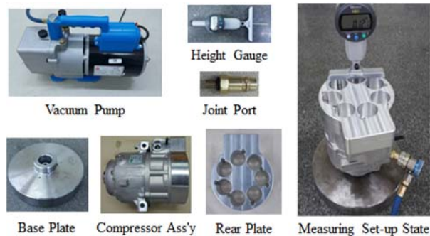
Fig. 5 Parts of vacuum type top clearance measuring.
