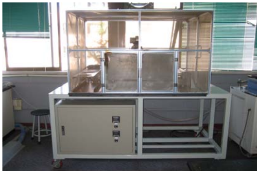
Fig. 2. Photographs of microwave-hot air hybrid drying system.
