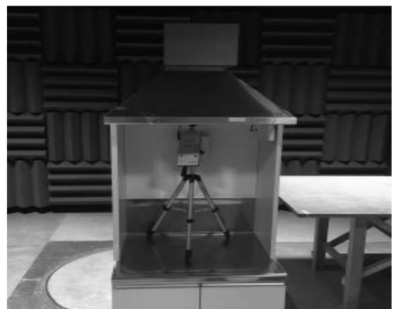
Fig. 3. test environment for noise reduction of range hood by Active Noise Controller.
