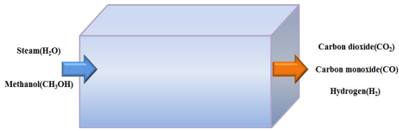
Fig. 4 Reaction principle of Steam-Methanol reformer
