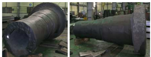
Fig. 10 Final forged hollow main shaft after flange die forging
